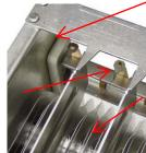
Be sure to coat corners & sides with cleaner, as well as both sides of all fins. Allow product to soak for 5 - 10 minutes. After rinsing a 2nd application may be needed for heavy soil.
