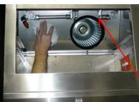
EVERY 30 DAYS, remove all 3 filters. Use an approved cleaning solution, or the Foaming Crystal Cleaner & a clean sanitized towel to thoroughly clean the inside of the hood
