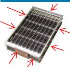
Place on drain board ... spray FOAMING CRYSTAL cleaner so as to cover all surfaces of fins & frame, ensuring all brass fittings are also covered ... flip over & repeat on the other side.
