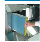
FILTER CANNOT BE CLEANED ... DO NOT ATTEMPT TO. CHARCOAL FILTER must be replaced about every 30-45 days, or as needed ... PO-VH filter P/N - 30248 ... OVH-10 filter P/N -31963 (Keep a back-up filter on-hand at all times). Remove filter by pulling straight out & discard. Place a NEW filter into hood. NOTE air flow arrow. Record date on label.
