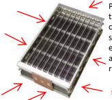
Place on drain board ... spray the FOAMING CRYSTAL cleaner so as to cover all surfaces of fins & frame, ensure all brass contacts are also covered ... flip over & repeat on the other side.
