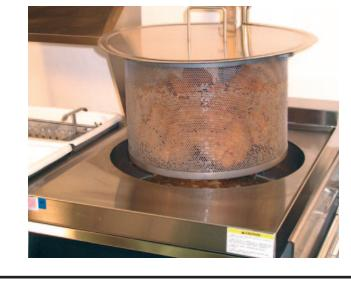
When the cook cycle is complete, an alarm will sound ... the basket will automatically return to the <u>UP</u> position. Allow product to drain.
