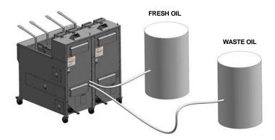
**GBF-80G Multi-well fryer** units can be purchased with *optional* factory-installed capability to be connected directly to a *customer-provided* bulk oil management system, which can either deliver fresh oil or handle waste oil disposal. Units can be ordered with either or both features.
