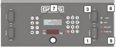
8. Place the **HEAT** switch **(3)** in **ON** position & fryer heating is energized. The **HEAT** light **(8)** will turn **ON** ... ignition sequence begins ... gas mixer/blower starts & burners ignite to begin heating oil to the setpoint temperature. Combustion noise should be noticeable.
