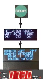
After selecting a *menu item preset,* or manually entering a *cooking time,* start the cooking cycle by pressing the **[START]** key once.
