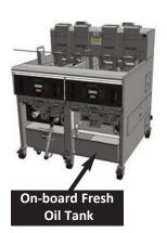
The on-board system pumps <u>fresh oil</u> from a <u>storage tank</u> located inside the right-hand cabinet. The tank has a capacity for approx. <u>70 lbs</u>. of liquid frying shortening & serves **all wells of the banked unit**. A suction pipe connected to <u>on-board top-off pump</u> reaches into tank at the front. Removable covers protect the stored oil from contamination.
