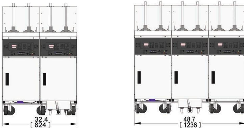
Add approx. 5" [127 mm] to width when equipped w/On-board Fresh Oil Supply option
