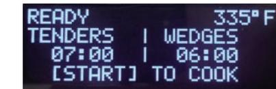
**COOKING TEMPERATURE, NAME, COOK TIME, STIR OVERRIDE & FISH FILTER** settings are shown on the *upper display*. **READY** message indicates that cooking oil is at proper temperature and fryer is ready for cooking.
