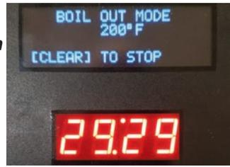
To exit **BOIL OUT MODE** before completion, press [CLEAR] + [4]
