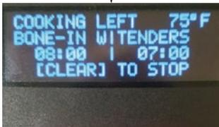
The *upper display* indicates the side that is cooking, and displays the temperature setpoint. **Timer Indicators** beside the *lower display screen* will indicate which timer is displayed.
