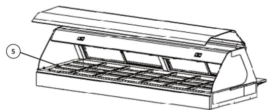
3. Install supplied <u>short pan support channels</u> **5** between each of the long support channels to create a pan grid to suit your particular need. Enough short channels are provided with each unit to create the grids shown in examples #2 & #3 on page 25.
