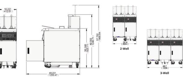
Construction: 16 to 20 ga. 430-series stainless steel; stainless steel tubular frame; (2) stainless Firebar heating elements
